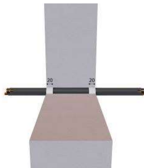
Figure A.1.4: Seal of a bunch of cables in a rigid wall.
