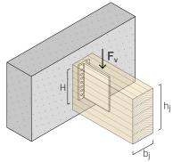
ALUMINI with SBD self drilling dowels and STA dowels
