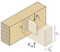
ALUMINI with SBD self drilling dowels and STA dowels
