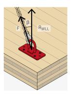
$\beta$  = lifting angle (angle between vertical axis and chain)  $R_{WLL}$  = working load limit for one anchor point
