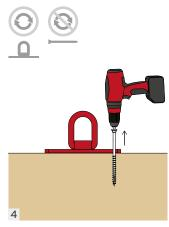
When lifting is complete, remove the screws and dispose of them. The screws can be used for only one handling cycle.
