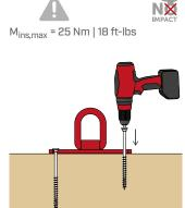
Length and quantity of screws depend on the type of application. Drive the screws in the holes provided, being careful not to overtighten them.
