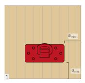
Read the instructions for use carefully and follow the directions. The positioning of the plate on the timber element must comply with the minimum distances.
