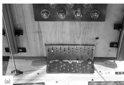
Samples at the end of cyclic tests: tension (a), shear (b) and 45^\circ (c) (partial fastening).
