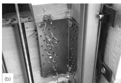
Samples at the end of cyclic tests: tension (a), shear (b) and 45^\circ (c) (partial fastening).
