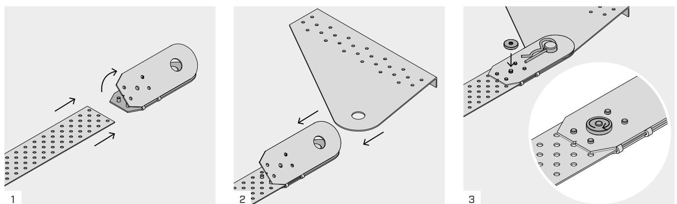
Open the end element and insert the perforated steel strap.
