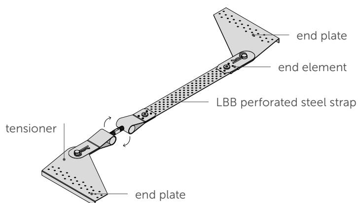
Use the tensioner to regulate the length of the bracing system.
