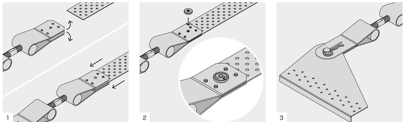
Open the tensioner and insert the perforated steel strap.
