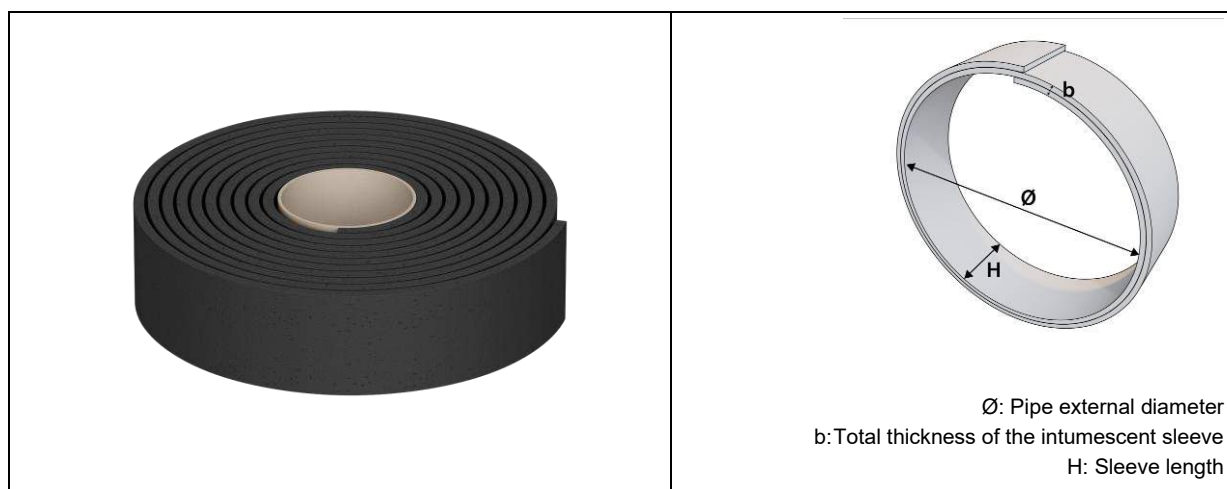
Figure B.1: General view of FIRE STRIPE GRAPHITE PRO (roll and preformed) and dimensions of the installed sleeve.
