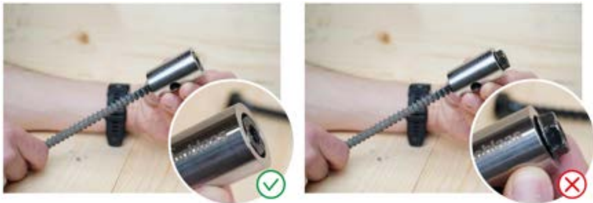
Figure 32. Real examples of visual inspections of used screws with gauge JIG REUSE. Straightness check passed, thus absence of significant plastic deformation (left). Straightness check NOT passed, screw to be discarded (right).
