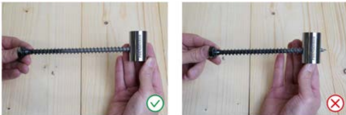
Figure 33. Real examples of visual inspections of used screws with gauge JIG REUSE. Thread wear check passed (left). Thread wear check NOT passed, screw to be discarded (right).
