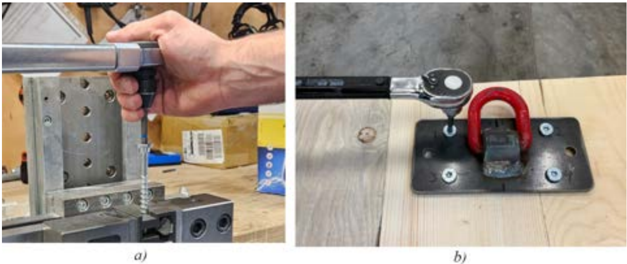
Figure 22. Tightening tests of HBS P10 screws: a) rigid thread fixing (pure screw torsional strength) and b) real installation condition using a thick steel plate (applicable torque in-use).
