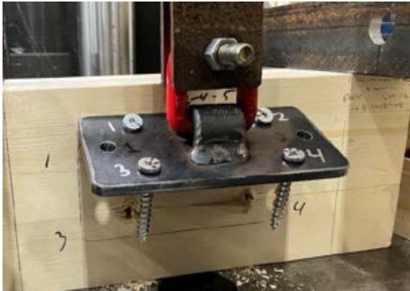
Figure 17. Pure shear tests at 0° after failure. Most specimens with HBSP1080 screws failed by withdrawal of the two lower screws, allowing the plate to rotate and the upper screws to deform.
