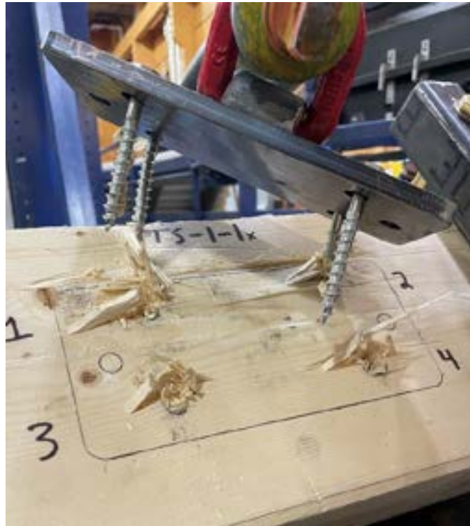
Figure 15. Combined tension-shear tests at 45° after failure. Most specimens with L=80mm (3 1/8") screws failed by withdrawal of the downhill screws, causing timber splitting and plate rotation, which then led to deformation of the uphill screws and further splitting.
