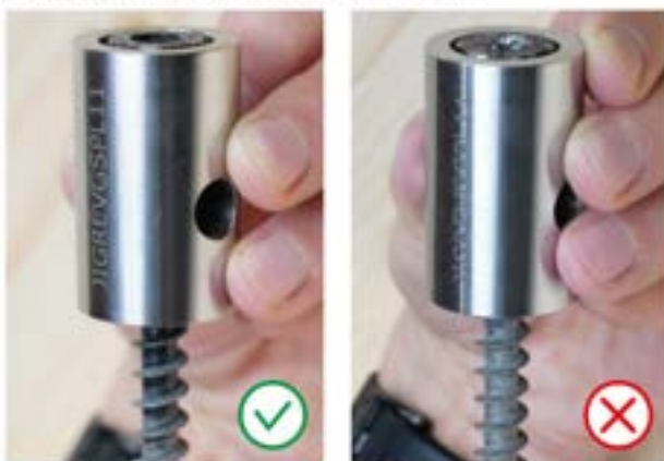
Figure 43. Real examples of visual inspections of used screws with gauge JIG REUSE. Number of uses check passed (left). Number of uses check NOT passed, screw to be discarded (right).
