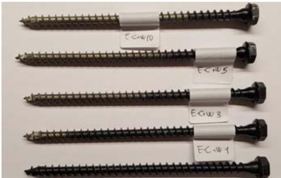
Figure 40. Screws after 1, 3, 5, and 10 insertion-withdrawal cycles, showing the progressive wear-off of the Ecoat + Wax coating.
