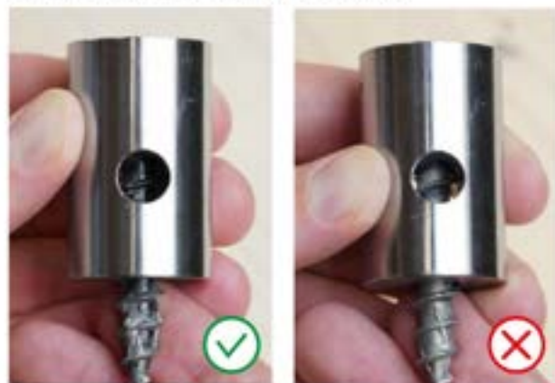
Figure 43. Real examples of visual inspections of used screws with gauge JIG REUSE. Number of uses check passed (left). Number of uses check NOT passed, screw to be discarded (right).
