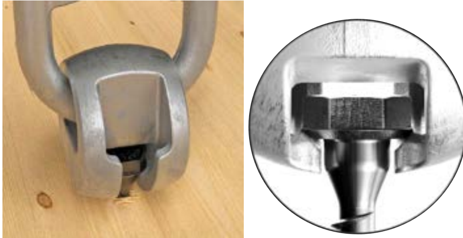
Figure 37. Renderings of VGS PLATE in application with the WASP lifting hook (left). Front view showing how the conical washer beneath the hexagonal head allows the screw to seat perfectly in the countersunk slot of the hook (right).
